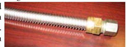
leak. Moving an appliance can cause failure of one of these older weaker flexible connectors. It is recommended that these older connectors be immediately replaced.
